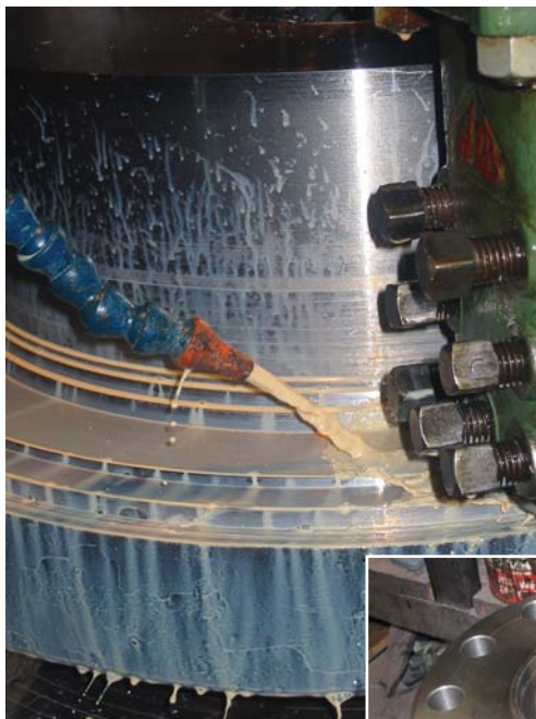
Large agitator couplings being manufactured to tolerances of less than 0.01mm for accuracy and control.
