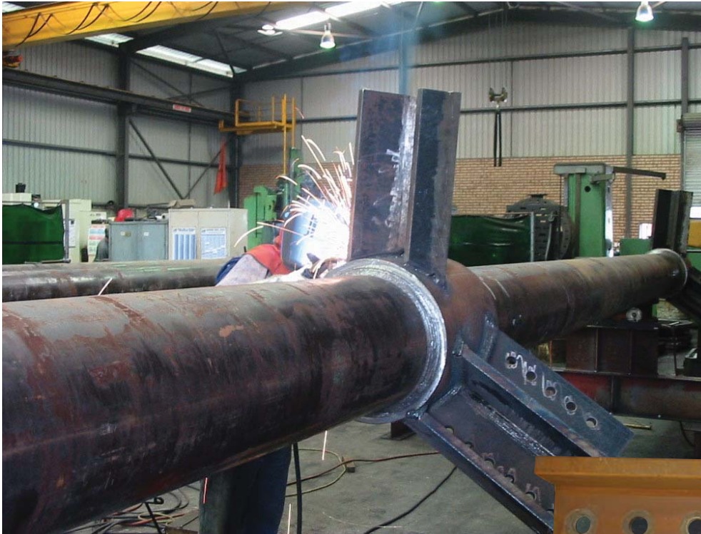
500mm nominal bore schedule 80 pipe shaft in production. Shaft length exceeds 20 metres
