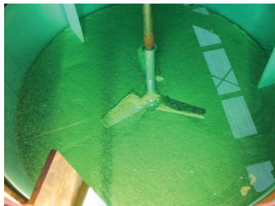
Solid suspension test work on Copper leaching application.
