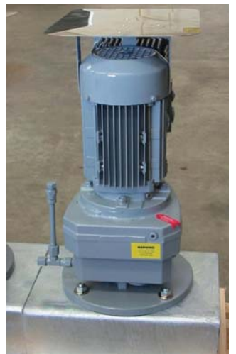
Series 1000 with weather protection and VVVF control
