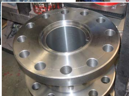
Large agitator couplings being manufactured to tolerances of less than 0.01mm for accuracy and control.
