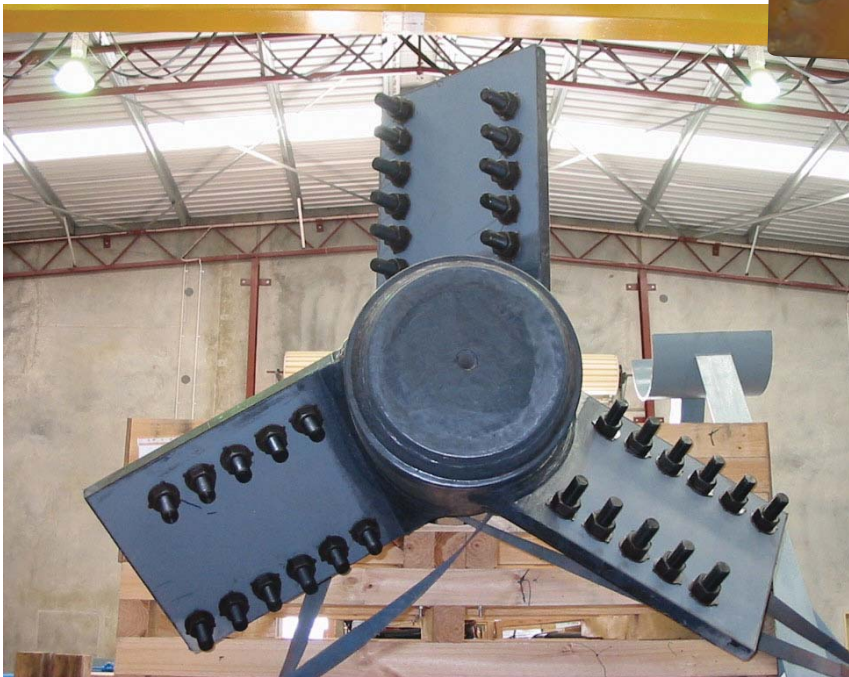
NDT inspection on reinforced impeller hub before magnetic particle testing and final coating
