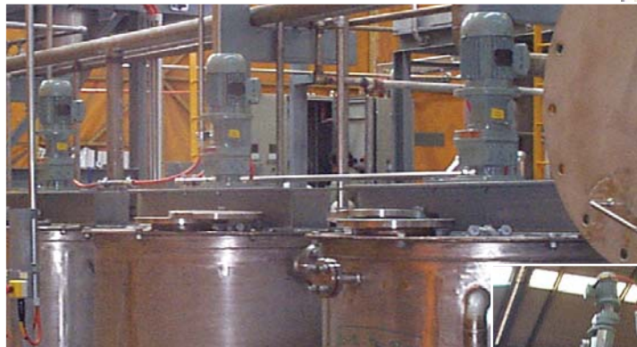
Series 1000 units on paint blending duty
