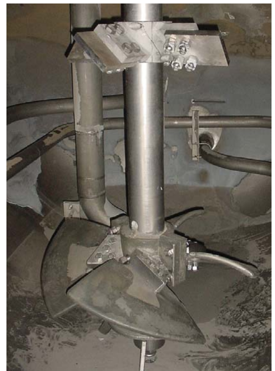
Large HA 735 impeller in a high pressure, high temperature autoclave
